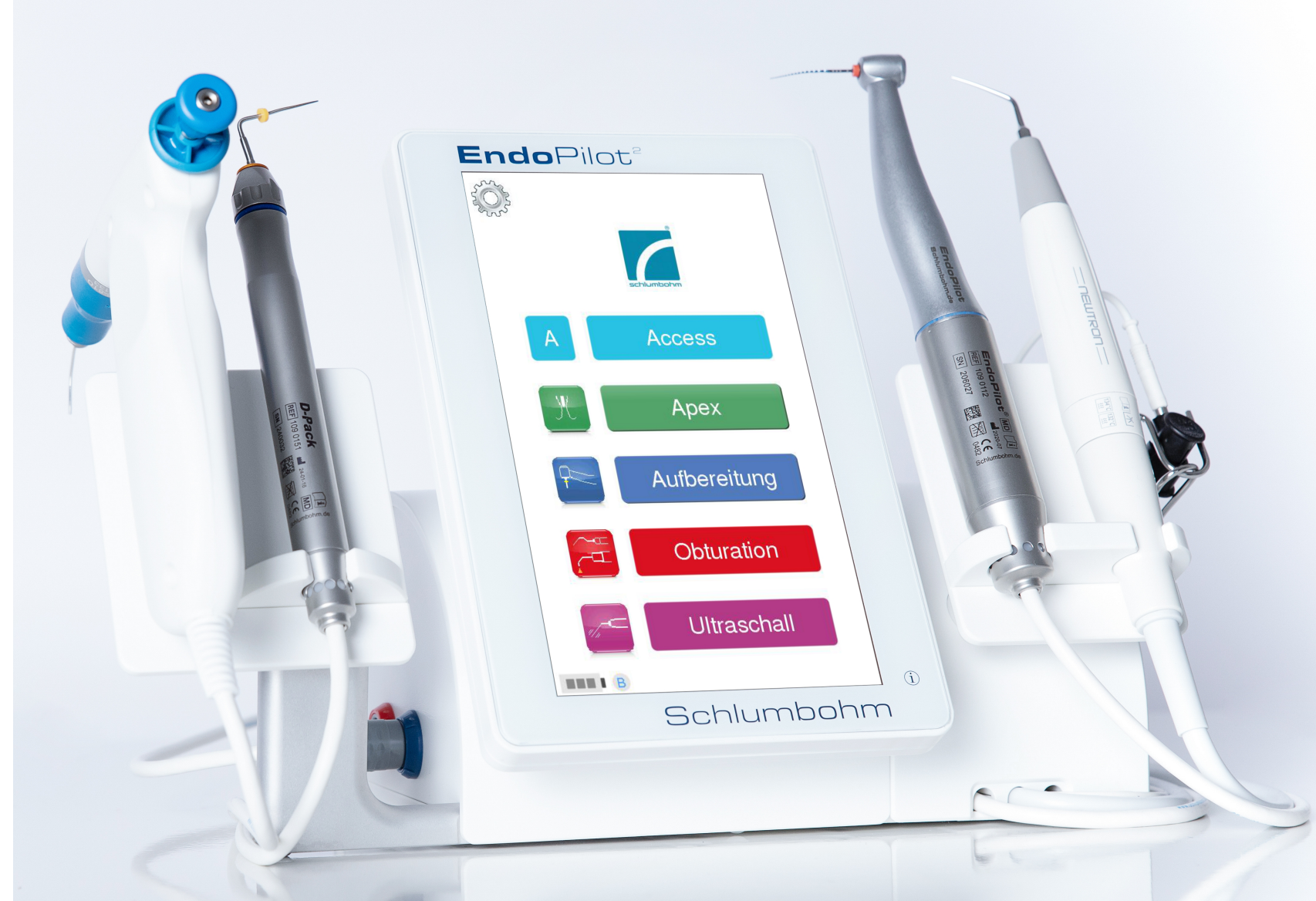
Fig. 3: Schlumbohm EndoPilot with prototype software to measure dentine impedance during access preparation and automatic reduction of bur speed in thin dentine zones to avoid perforation.
