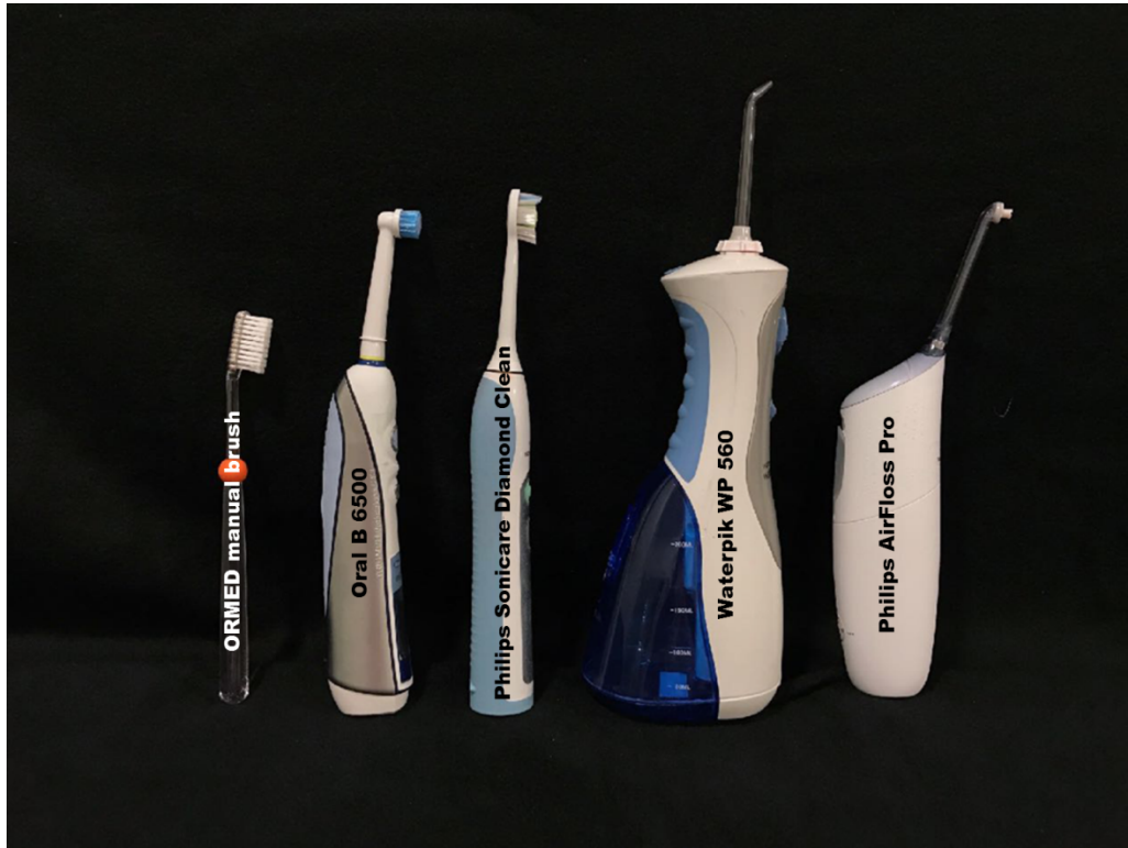
Figure 1: Tested brushes (from left to right): ORMED manual brush, Oral B 6500 powered toothbrush, Philips Sonicare Diamond Clean powered toothbrush, Waterpik WP 560 jetting device, Philips AirFloss Pro jetting device.
