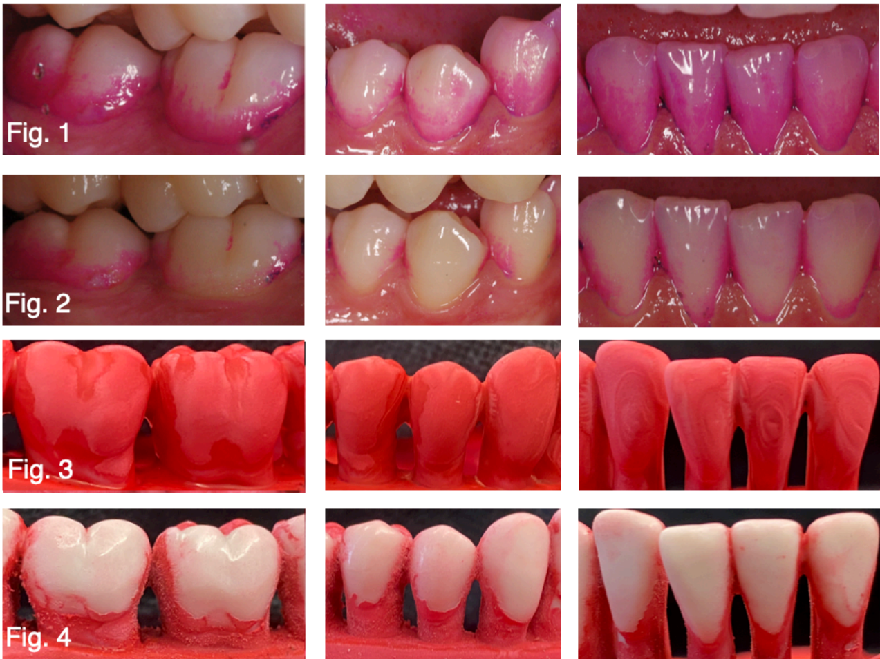
Fig. 1-4: Stained clinical plaque after 3-day plaque regrowth (Fig. 1); stained clinical plaque after brushing for 20 s with force 3.5 N (Fig.2); stained organic plaque simulation on KaVo teeth (Fig. 3); stained organic plaque simulation after robot brushing for 20 s with force 3.5 N (Fig. 4)
