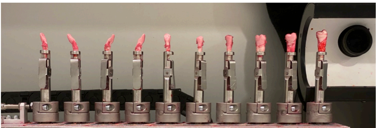
Fig. 6: Automated Plaque Planimetry (APP); teeth covered with organic plaque simulation after brushing, site by site rotating in front of the HD focusing analysis camera followed by computer-assisted processing of plaque percentage per each single field
