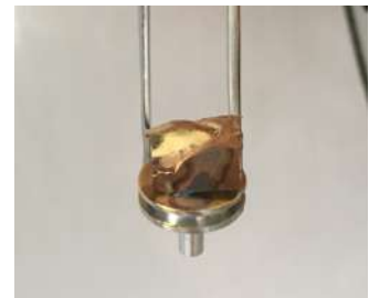
Figure 15: A sputtered tooth replica glued on a pen holder for SEM investigation.
