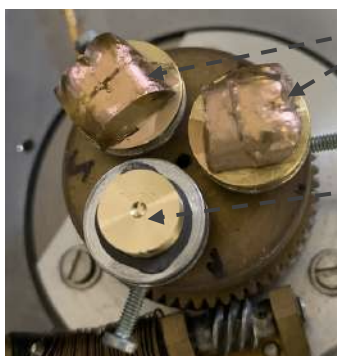
Figure 20: Two replicas (pre and post) and the calibration block together on the sample table.
