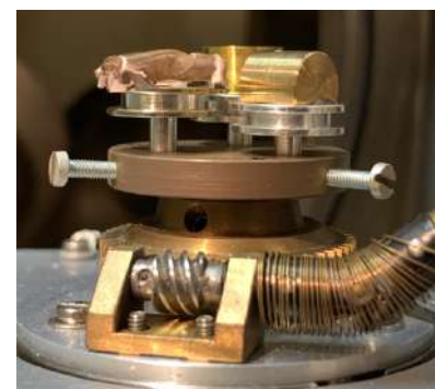
Figure 21: The two replicas and the calibration body were adjusted to the same height.
