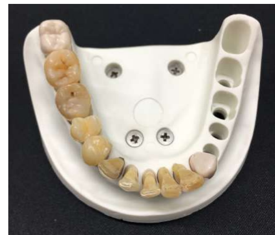
Figure 10: Human tooth model B – nine human teeth of different ages were aligned in anatomical position to be brushed with the Jubilee toothbrush.
