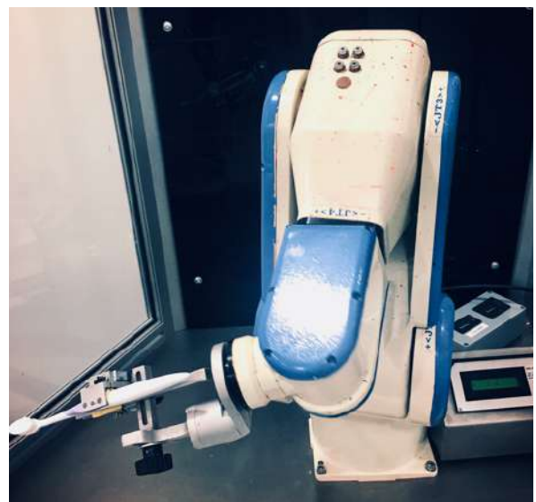
Figure 11: The validated six-axis robot (FS02N, Kawasaki, Akashi, Hyogo, Japan) is holding the manual toothbrush "Jubilee Soft" with rigid neck and a flat trim.
