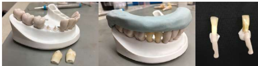
Figure 8: The tooth holder by KaVo is designed to simulate the physiological situation of a dentition ( eugnathia ) including the bony contour of the jaw. It has specially manufactured notches into which plastic teeth can be clicked. The silicone wall was used to ensure the position of the real teeth in the dental arch. Human teeth were polymerised on plastic pins and could thus be easily removed and repositioned from the model.
