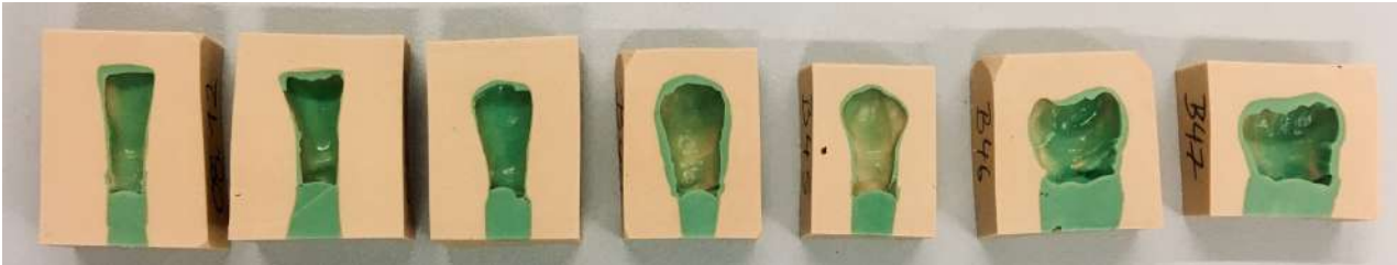
Figure 14: The green Affinis light body impressions were cut into flat squares and labelled with the respective tooth identification number. After 30 minutes of set-up time, the impressions could be cast with epoxy resin. In advance, the impressions were checked with stereo microscope for oil and cleanliness.
